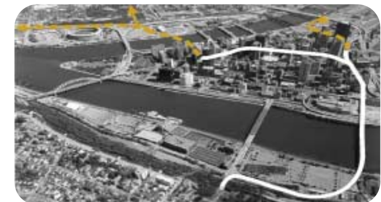
The Gateway alignment is deemed the most compatible with the City of Pittsburgh's plans for future development along the North Shore. This alignment also offers the least construction and property impacts of all of the alignments under consideration. The North Shore Connector will include five new "T" stations: the Convention Center Subway Station; a new inbound Gateway Center Subway Station with an entrance on Stanwix Street directly adjacent to Fifth Avenue Place; a subway station just west of PNC Park; an at-grade station at Steeler Way; and a station at the proposed Intermodal Transportation Center.
